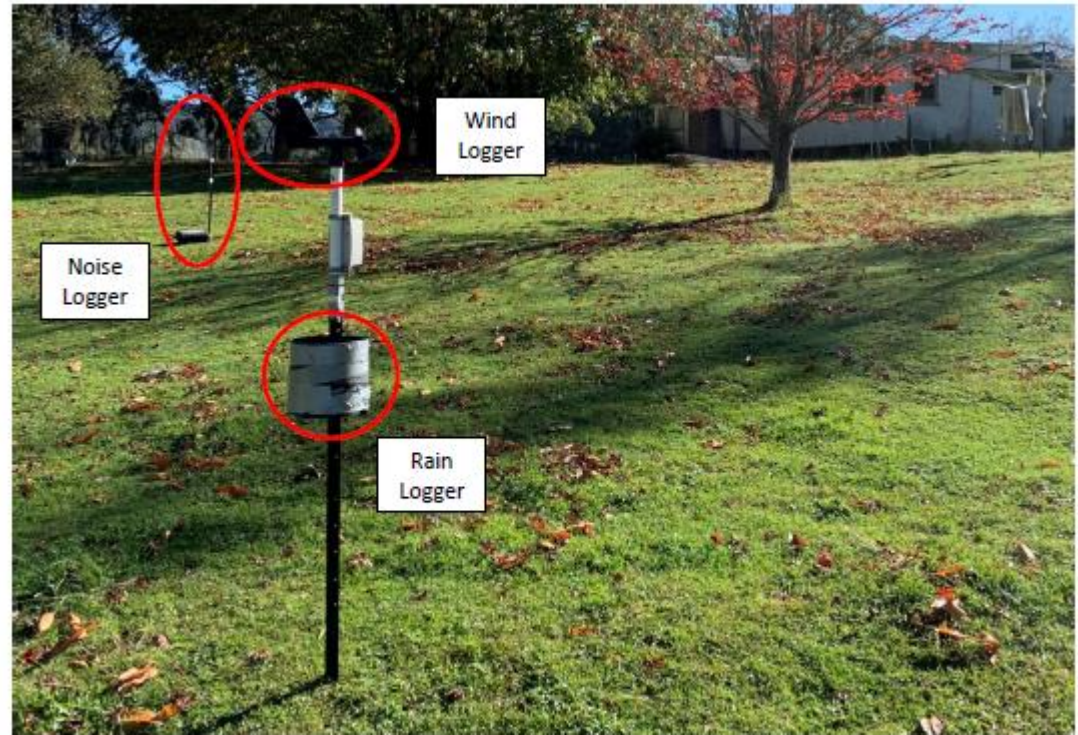
Typical Monitoring Setup
